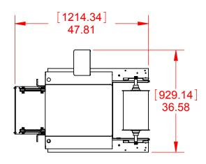
**DIMENSIONS ARE IN INCHES** PROPRIETARY AND CONFIDENTIAL TOLERANCES: FRACTIONAL: ±1/64 ANGULAR: MACH: ±1° TWO PLACE DECIMAL: ±0.010 THREE PLACE DECIMAL: ±0.003
