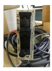
If the Red Error Light is OFF and the PLC is in RUN mode. The follow issues indicate that the program is corrupt
