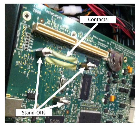
Notice the contacts on the back of the Ethernet Board (below). These will line up with the contacts on the Logic Board.
