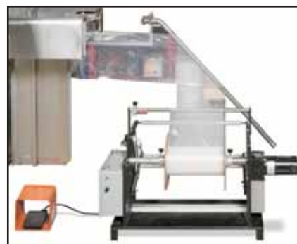
Controlled tension with driven unwind stand to handle large diameter rolls for longer production runs.
