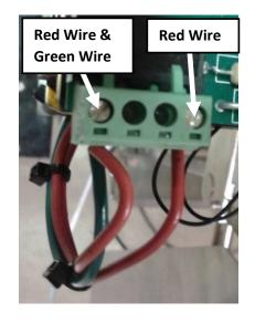
Plug in cables, and dress Transformer wires as shown.
