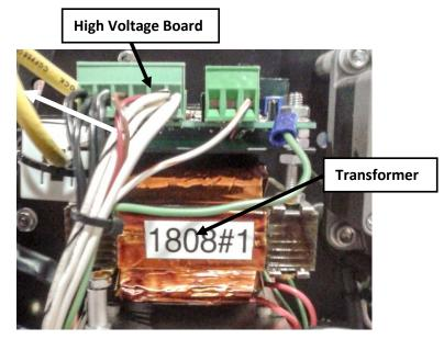
Unplug all four cables from **High-Voltage Board** (J1 through J4), & disconnect Ground Wire:
