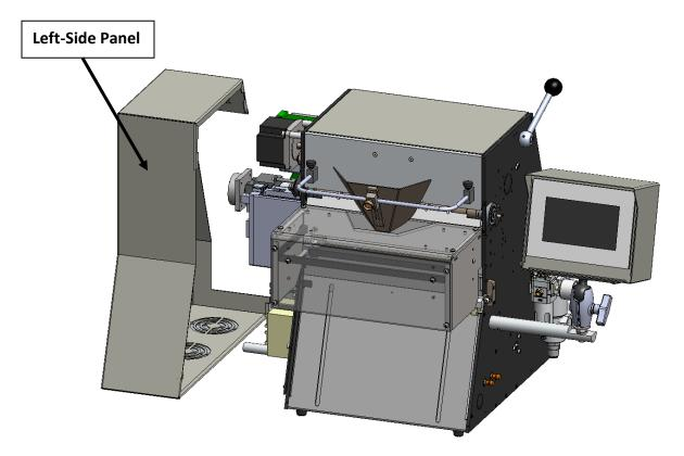
Unscrew and remove the two #8 Socket Head screws on each Side Frame. Loosen the top one on each side.
