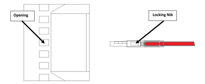
Reinsert the connector into the PLC, pressing it into place until the tabs snap back up, securing the connector.
