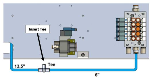
Connect blue tubing to the Valve, Manifold, Tee, and Load Shelf Cylinder as shown.
