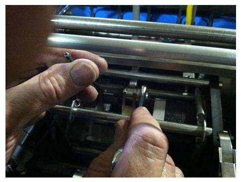
Loosen the Nut and remove Shoulder Bolt.
