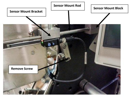
It will be necessary to remove the bottom screw in the Bag Blow-Off Block, and pivot the Block to allow room for the Sensor to be installed.
