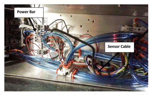
Attach Grey connector with Black Wire (provided) to Power Bar metal slide with the metal side facing upward.
