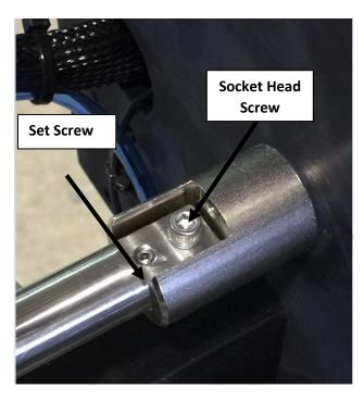
Loosen the Socket Head Screws on both Guide Rod Holders.
