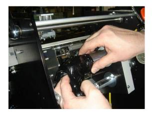
Unlatch the Printhead assembly and carefully tilt back the head to the fullest backwards position, not allowing it to drop.
