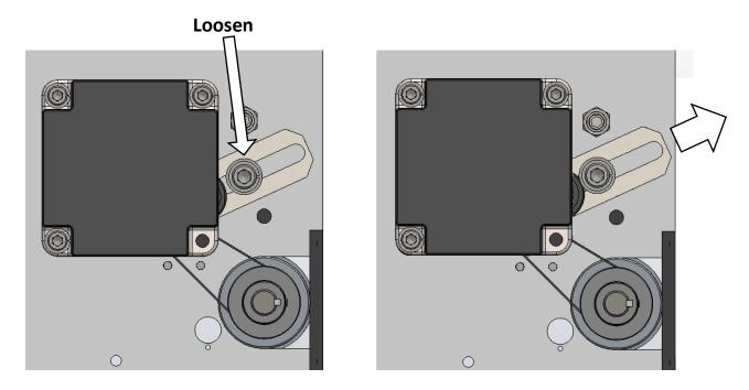
Remove worn Drive Belt. Install replacement Drive Belt.
