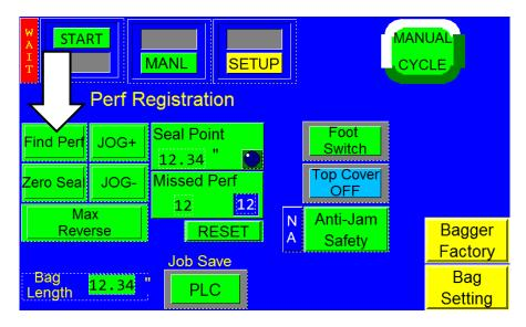
Press Find Perf. The Bagger will advance the bag until it stops on a perforation.
