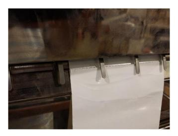
Press and hold "JOG-" until the perforation is under the fingers.
