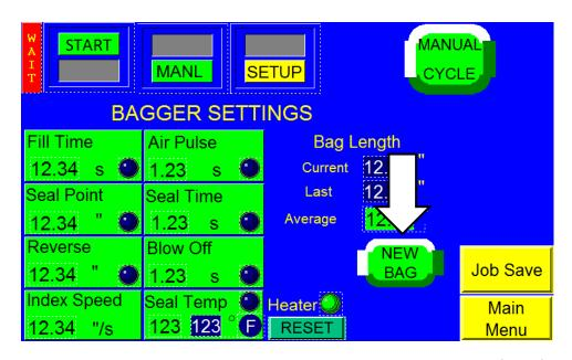
Press "NEW BAG". Press "MANUAL CYCLE" until Bag Length Current/Last/Average is about the same numbers. This usually takes 4 to 5 cycles.
