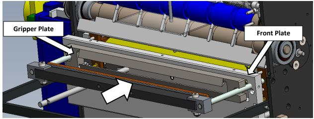
Slide Gripper Plate and Front Plate back to line up with Pivot Pin Hole.
