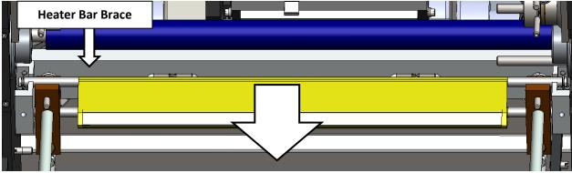
Slide the heater Bar Brace out.
