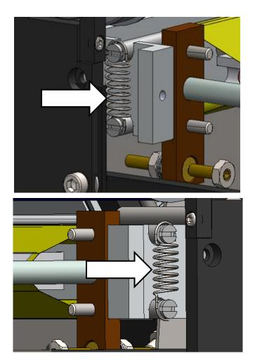
Remove the right and left Springs that hold the PTFE Sheet Shafts in place.
