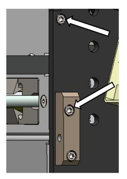
Remove the two #8 Socket Head Screws on the Right side of the Bagger.
