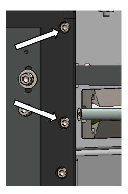
Remove the two #8 Socket Head Screws on the Left side of the Bagger (one may have a green ground wire attached to it).
