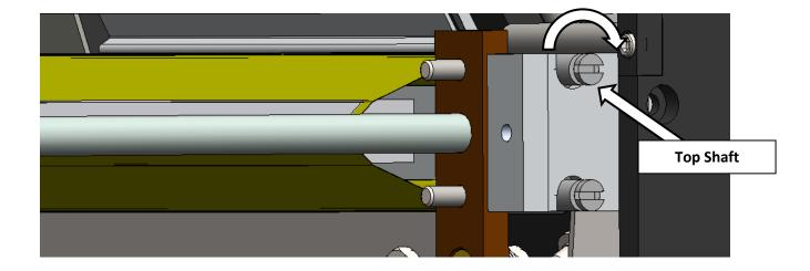
The Top Shaft is the Supply Shaft, so wind the PTFE onto the Top Shaft.
