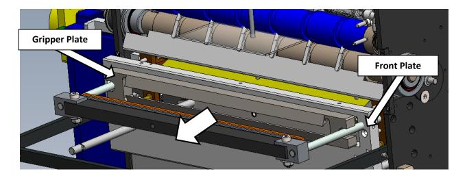
Slide the Gripper Plate and Front Plate out.
