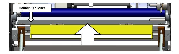
Slide Heater Bar Brace back into place.
