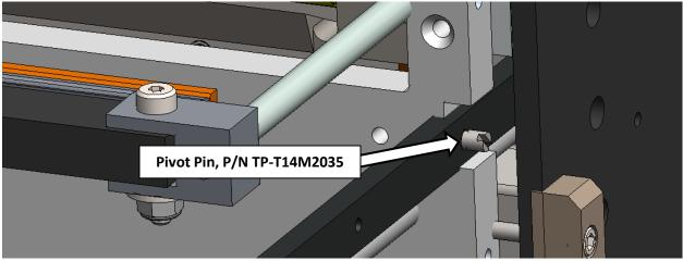
Carefully pull Front Plate and Lexan Guard Bracket out and unscrew the Pivot Pins on both sides of the Front Plate.
