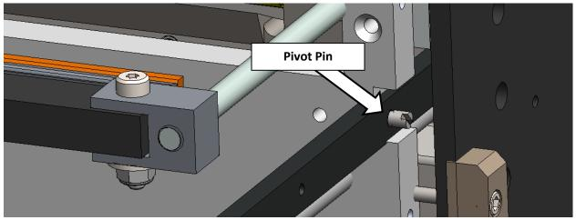
Insert Pivot Pin and screw in. (BOTH SIDES). Slide Gripper Plate and Front Plate back into position.
