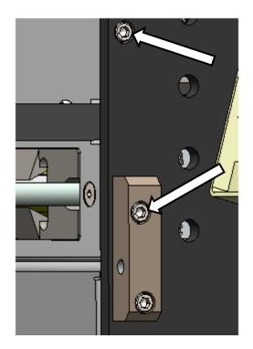
Replace #8 screws on both sides. Reconnect Ground Wire.
