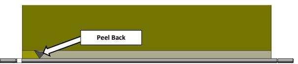
Remove adhesive backing cover, and position shaft on PTFE Sheet, then roll on.
