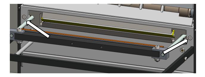
Replace the 2 Flat Head Screws into Front Plate. It may help to reach behind and push the Heater Bar Brace forward to the Front Plate.
