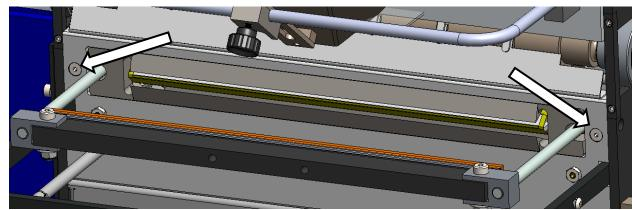
Unscrew and remove the two #8 Flat Head Screws from the Front Plate.
