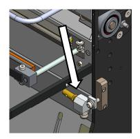
Remove Button Head screws; remove Lexan Cover. Remove Bag Blow Off.
