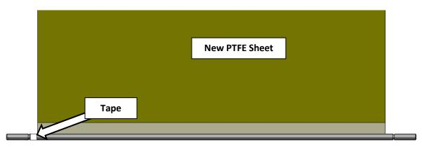
Line up and center the new PTFE Sheet with the tape marks.
