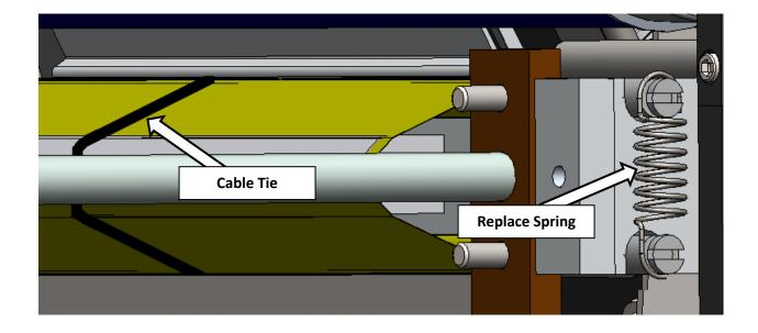
Put a Cable Tie around both PTFE Shafts to hold them in place while replacing the Springs. Remove Cable Tie after Springs are in place.
