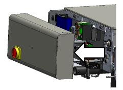
Locate Transformer and High-Voltage Board.
