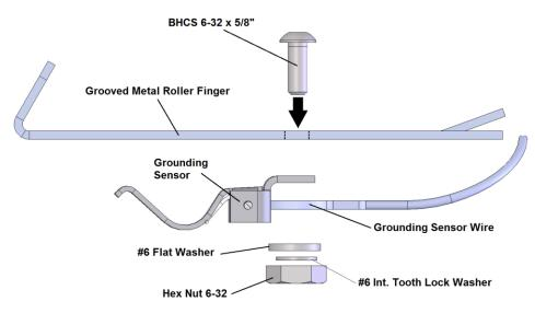
Align the Grounding Sensor so that it is square with the opening and touching the Steel Roller.
