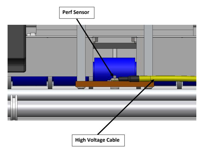
Adjust the placement of the Perf Sensor so that it is in contact with the Steel Roller.
