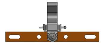
The Perf Sensor is connected to the High Voltage Board using the High Voltage Cable, which is secured under the Hex Nut of the Perf Sensor assembly.
