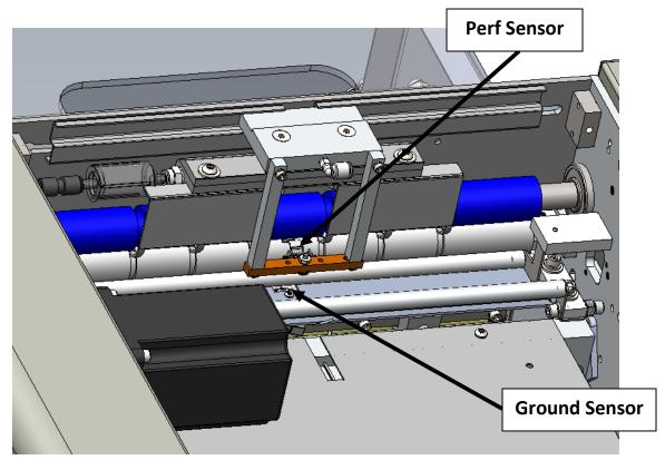
Functionally, the Perf sensor is connected to the output of the High Voltage Printed Circuit Board (PCB) and conducts the voltage to the Steel Roller. The Ground Sensor connects the Steel Roller to Ground, completing the circuit.
