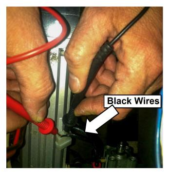
If the **Heater Cartridge** is good, your meter should read approximately 18 Ohms on a 110 Volt Bagger, and 60 Ohms on a 220 Volt bagger.
