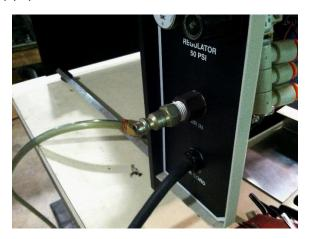
Remove the Stainless Back Cover by removing the screw on each side.
