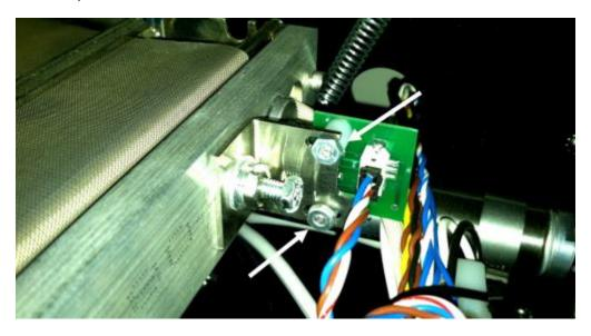
Install the new Anti-Jam Circuit Board, and tighten the Lock Nuts.
