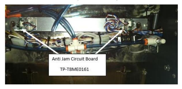
Unplug Pig Tail connector from the Anti-Jam Circuit Board you intend to replace.
