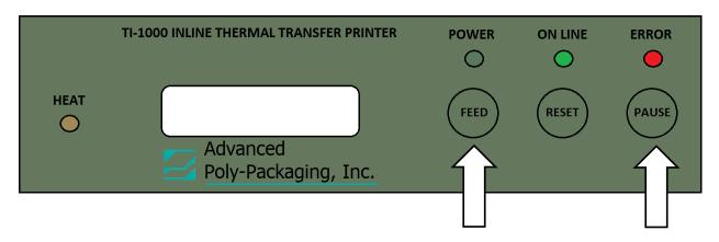
Turn power "ON" while holding the buttons. "DIAG V\_\_\_\_" will be displayed on panel.
