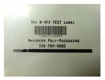
If one side of label is not printing clearly, loosen the Phillips Head Screw on that side, and move the Print Head slightly forward or backward. Tighten the Phillips Screw.
