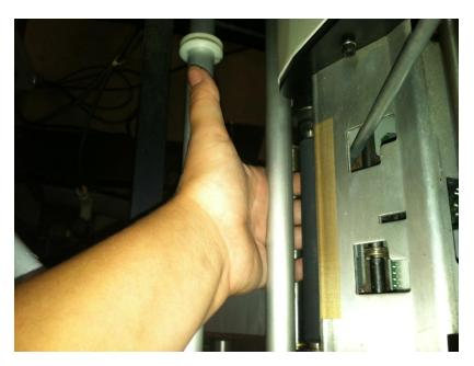
Carefully line up the 2 clearance holes with the 2 threaded holes in the Print Head. Carefully replace the 2 gold color Phillips Head Screws. Do not tighten.
