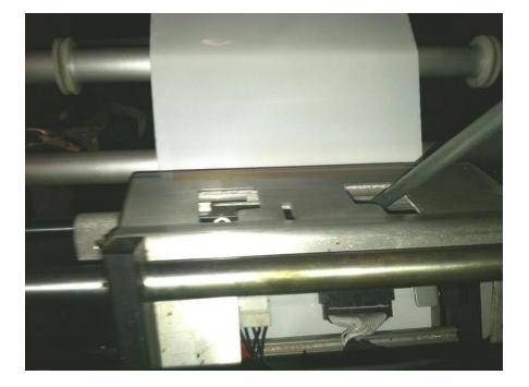
With a long Magnetic Phillips Screw Driver, remove the 2 Phillips-Head Bolts while supporting it underneath. Be careful not to round out the bolts when removing.
