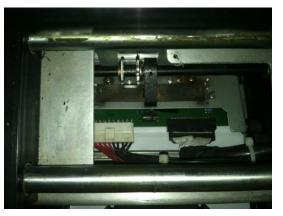
Remove Cover Plate from the top of Printer by removing the Phillips Head Bolt.
