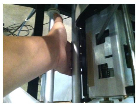
Carefully slide the Print Head under the Print Head Carriage. Do not let it drop or scratch the Pixel Strip on the bottom of Print Head.
