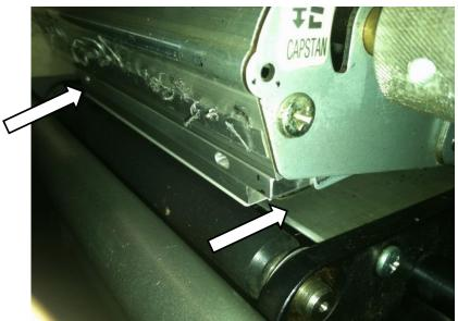
Carefully push both sides of the Print Head back; lightly tighten Phillips Head Screws.
