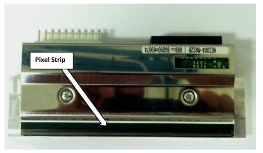
Carefully remove new Print Head from Bubble Wrap. Shown in the photo above is the bottom side of the Print Head. *Be extremely careful not to damage the pixel strip on the Print Head.*
