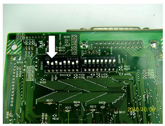
Note: Baud Rate is controlled by DSW 101, SW 2.
