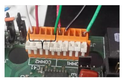
Connect the scale board programming port to COMM2 as shown in the picture:
