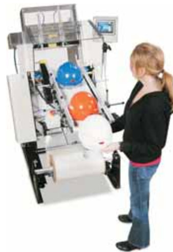
Debbie is packaging hard hats with an infeed conveyor.
