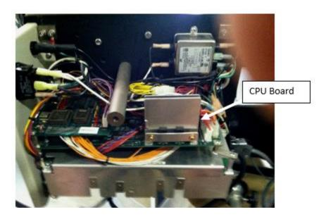
Remove the side cover to view the CPU
