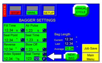
On the Bagger Settings screen, select "Seal Temperature".
