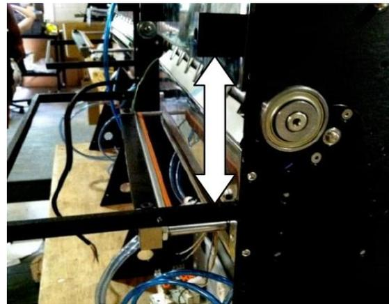
Distance from Perf Sensor to Heater Bar is longer.
