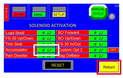
Press the Green Button next to Accumulator and assign a valve number for the Accumulator.
