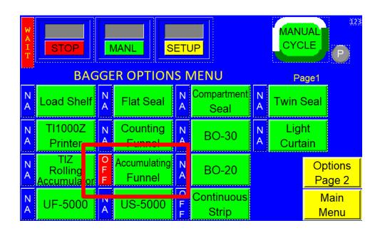
The Green Accumulating Button should display Red OFF to the left side of the button.
