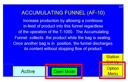
Press the Blue Closed Mode Button the switch to Open Mode
