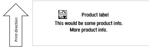
It prints from the bottom of the label to the top. The print head comes down on the bottom border of the label. Then it lifts up again at the top edge.
