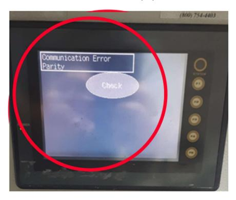
A communication error displayed on the Touch Screen normally is a result of a lost connection with the PLC in the bagger.
