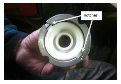
Put Nylon piece in #2. Note: the notches must line up.
