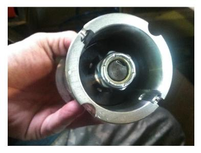
Thread on #5-¾" nut so that 2 threads are showing.
