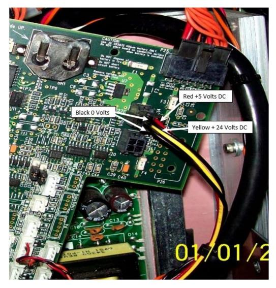
Turn Main Power off. Disconnect the Power Connector from the Logic Board. Measure the voltage between the Black and Red wires in the connector; it be +5VDC. Measure between Black and Yellow wires; the voltage should be +24VDC.
