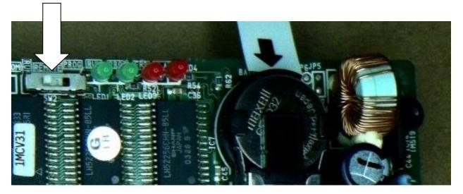
Turn power OFF and move mode selector switch to PROGRAM (far right position).
