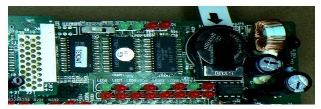
Carefully use a small screwdriver and remove battery; Replace with new one (NOTE + SIDE OUT).
