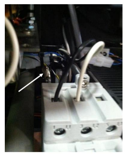
Loosen the Lock Nut then press down on the Lexan Cover; the Switch should light up when pushing down. If not, turn the Bolt/Switch in until it lights up when pushing Lexan down.
