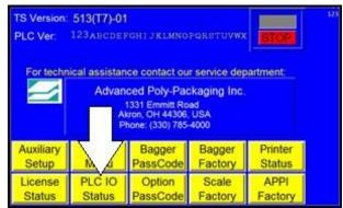
Enter Pass Code "1001", and press ENT. Press PLC Info. This will bring up the PLC I/O Screen.
