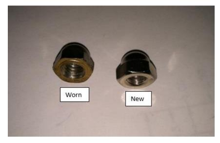
If Acorn Nuts are worn, order Replacement Part # TP-101131 (Nut, Acorn Brass Nickel Plate)
