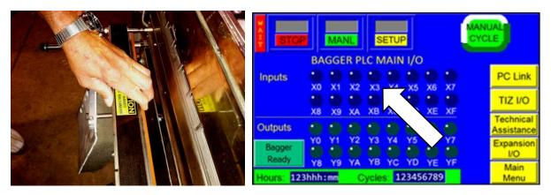
While squeezing The Pressure Bar, verify that X3 or X4 goes Out.
