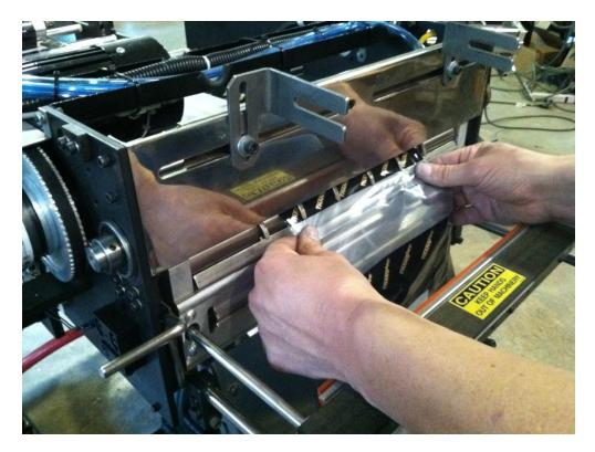
With the Jaw closed, see if you can pull a bag out. The bag should almost tear.
