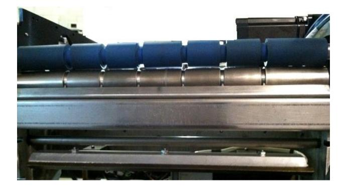
If Rollers are not parallel, you will need to adjust the Latch Lock Blocks.
