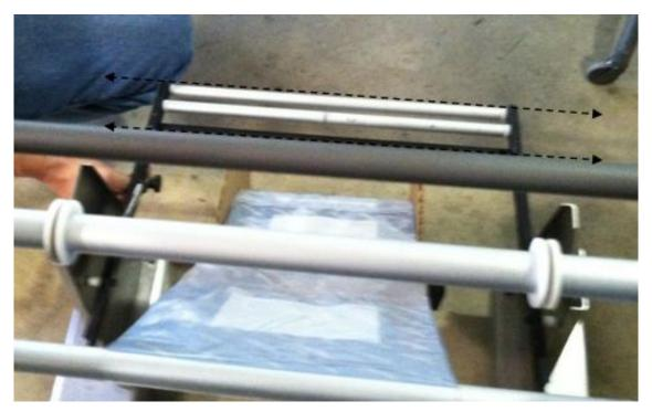
If the shafts are not parallel, loosen 2 Socket Head Bolts on Dancer Frame and move Dancer Frame Fore or Aft to parallel Dancer Roller with Bagger Shaft.
