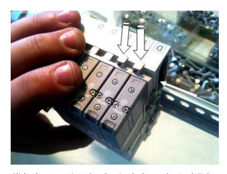
Slide the new Air Valve On. Push down the Lock Tabs.
