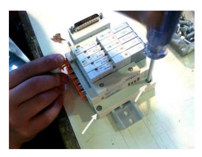
With a Phillips Screw Driver loosen the two screws on the Manifold Block.
