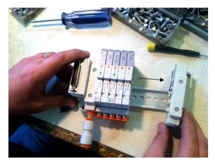
Slide the Manifold Block off.
