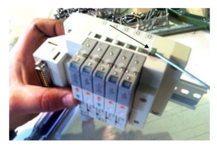
With a small Screw Driver gently lift the Lock Tab.
