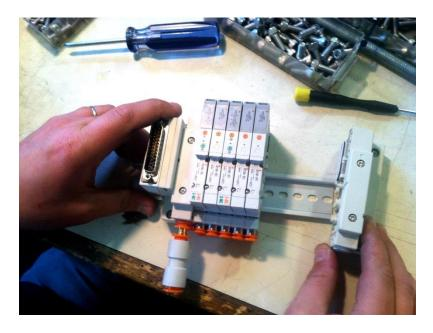
Slide the Manifold Block on.
