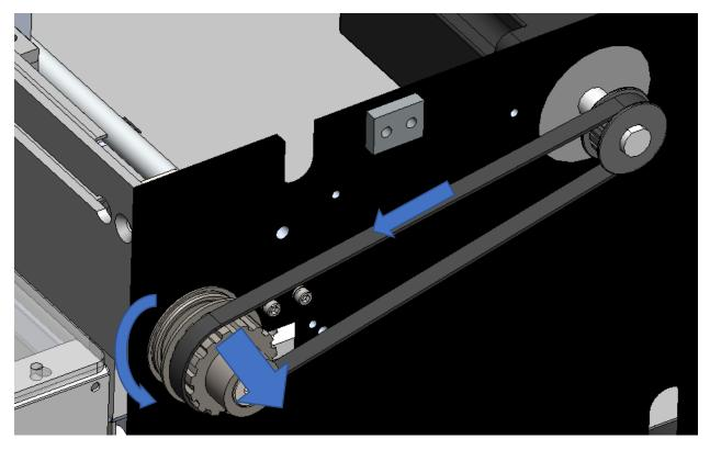
Slide belt off **Drive Pulley** while rotating, and remove from **Motor Pulley**.
