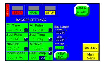
The typical temperature is setting is between 360°F and 440°F (182°C to 226°C) depending on film thickness.
