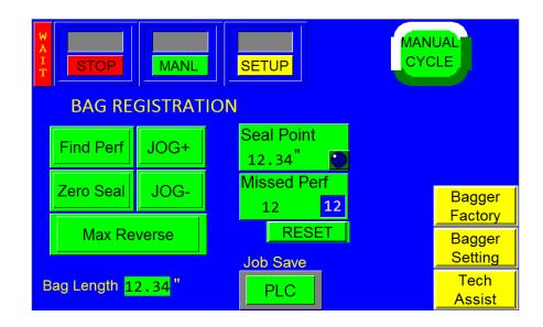
To determine if the **Seal Point** is registered, set the **Seal Point** setting to the lowest possible setting. Then press the **"Manl"** cycle button or press the foot switch. The bag should move so that the perforation is approximately **1/8**" from the center of the heater bar. If the bag perforation is not approximately **1/8**" from the perforation, perform the following procedure carefully. If these steps are performed out of order, the bagger will not function properly.
