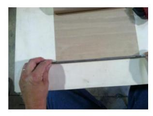
Lay **Heater Plate** on a flat surface so the side plates stick up. Lay PTFE sheet over the Heater Plate so that the shafts are parallel to the plate and the PTFE will roll on the outside of the shaft when reattached.
