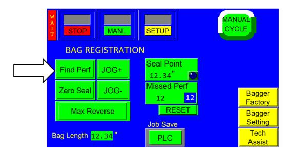
Press Find Perf. The Bagger will advance until it stops on a perforation.
