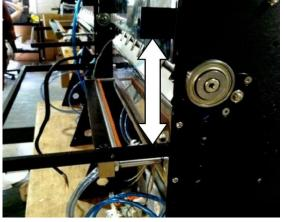
Distrance from Perf Sensor to Heater Bar is shorter. Distrance from Perf Sensor to Heater Bar is longer.
