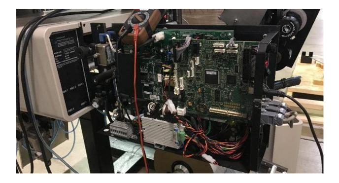
Locate the Ribbon Sensor plug. It will have the four wires, and will also be marked RIBBON SENSOR.
