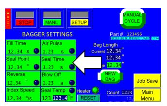
Typical Seal Time with temperature set to 400°F is 0.3 seconds for thinner bags (1.5 mil), 0.4 seconds for medium thickness (2 to 3 mils), and 0.7 seconds for heavier thicknesses. However, the set temperature will affect the Seal Time.
