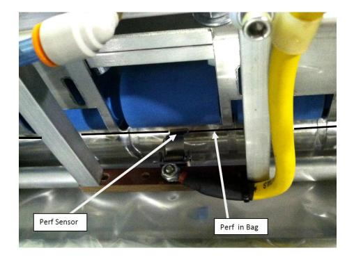
Press and hold JOG+. Until the Perf is Center in the Heater Bar Gap
