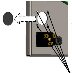
Using a Utility Knife and working from the inside, cut out a circular opening for the Panel Connector. It will also be necessary to punch out the four (4) mounting holes in the Mylar overlay.
