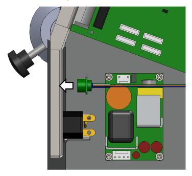
Secure the Panel Connector in place using four (4) 4-40 x 1/2" Machine Screws, #4 Lock Washers, and 4-40 Hex Nuts. The wires will be connected in the next section.
