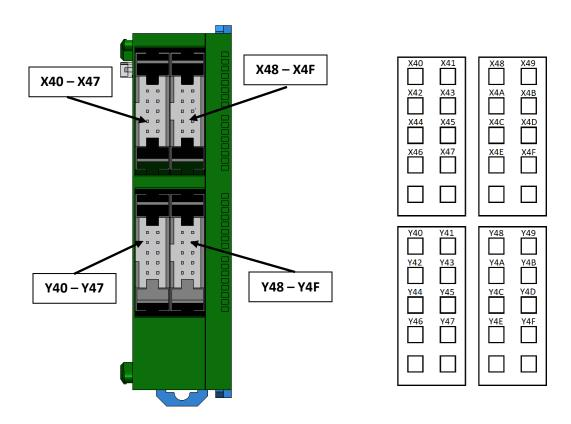
To connect the Relay Wire to the PLC Expansion, remove the Plug in the Y40 – Y47 position (Lower-Left) by pressing down on the tabs. When the Plug is free, insert the Crimp on the end of the Black/White/Yellow wire into the Y40 position (shown). Make sure the locking nib is facing the corresponding opening in the Connector Housing.
