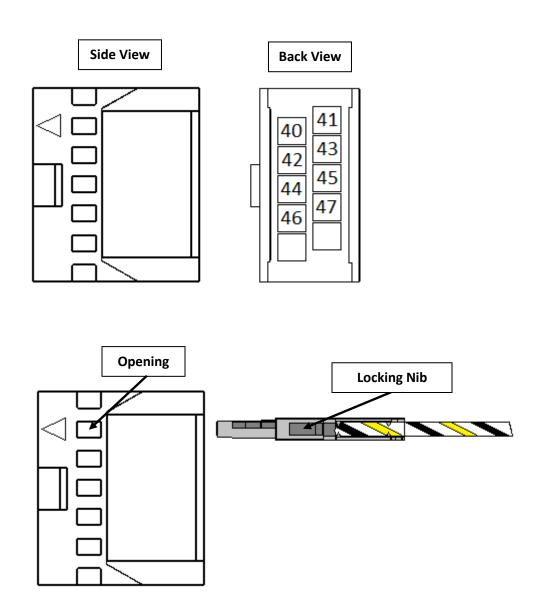
Reinsert the connector into the PLC Expansion Module, pressing it into place until the tabs snap back up, securing the connector.
