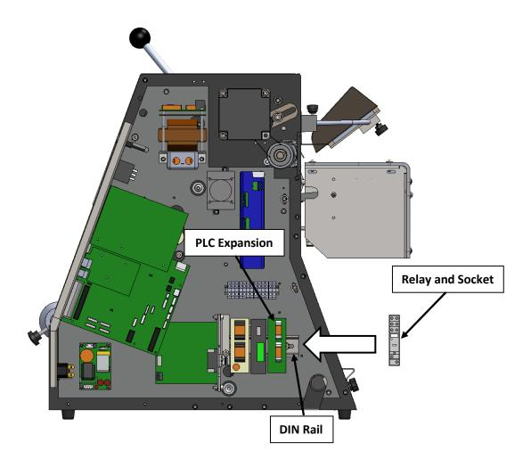
There are two wires attached to the Relay Socket that must be connected to the T-375:
